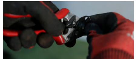
3. Ajuster la tension.
