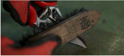
1. Use a metal brush to remove dirt & rust from the cutting head.
