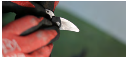
8. Use adjustment key to scrape dirt and rust from blade and anvil blade.
