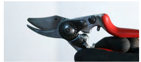
6. Blade crossing should be between 1/2 & 2/3.
