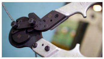
Cable cutter gearing mechanism
